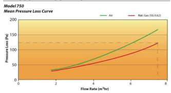
Pressure loss is made of two components pneumatic pressure loss (created by small passage ways and the movement of gas through the meter) and mechanical pressure loss a result of moving components.
