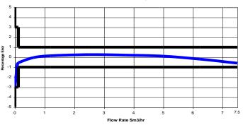
The 750 is built for a service life of many years and to an initial accuracy of better than +/- 0.75% error.
