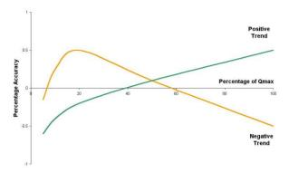
The 750 high resolution adjustable tangent allows precision fine tuning of both meter Accuracy and accuracy trend (accuracy at Qmax relative to 20% of Qmax). The ability to set timing is an important feature of the meter. Like a well tuned engine it assures smooth operation and reduced wear.
